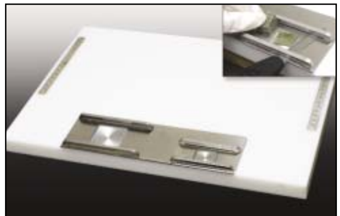
Image 3_ Specially designed dissecting board, with recessed areas and scalpel blade guides for trimming tissues to desired thickness.
